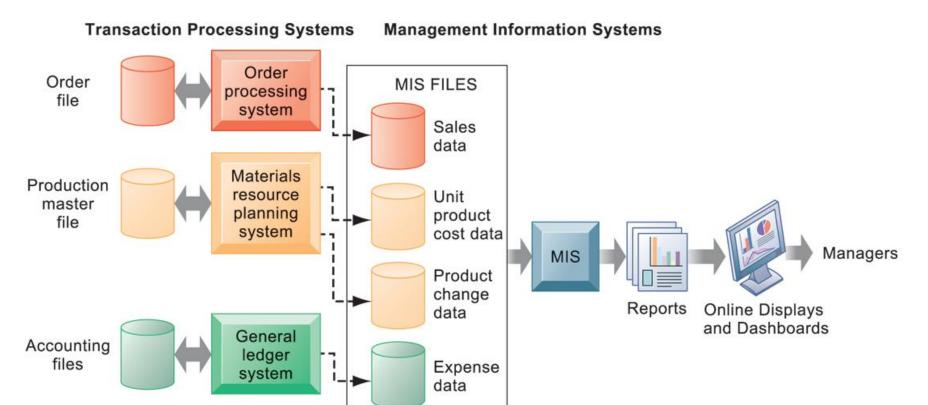
In the system illustrated by this diagram, three TPS supply summarized transaction data to the MIS reporting system at the end of the time period. Managers gain access to the organizational data through the MIS, which provides them with the appropriate reports.
