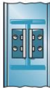
typical “pin-supported” connection (metal) (a)
