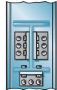
typical “fixed-supported” connection (metal) (b)
