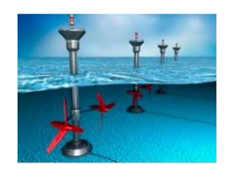
This is another form of hydro energy that uses twice-daily tidal currents to drive turbine generators. Although tidal flow unlike some other hydro energy sources isn't constant, it is highly predictable and can therefore compensate for the periods when the tide current is low.
