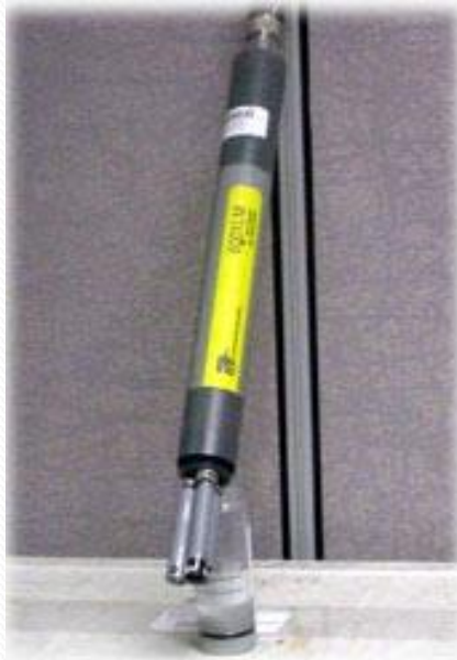
Water-quality meter to measure multiple parameters in the field.
